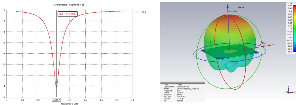
Fig 2: Reflection coefficient and Radiation pattern of the circular patch antenna.
